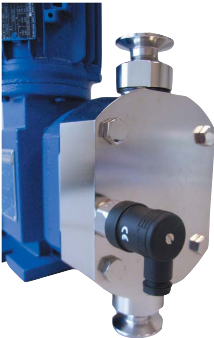
Electropolished pumphead Ra <0,8µm with pressure switch for diaphragm monitoring service
